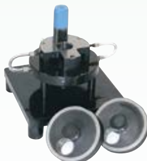
ピッチ測定台 For measuring pitch
